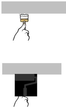
We recommend applying FarbTon clay paint with a brush. To obtain a uniform paint coat, apply the paint in changing directions. Trace a flat eight with the brush to avoid brush strokes. With this method, you can see that it is handwork, it gives the surface a vital look, however.
